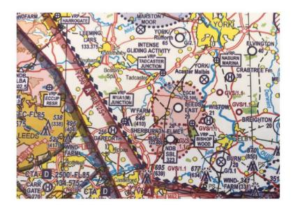
Sherburn has three runway orientations, as depicted below on the accordon a chart The most commonly used runway is the hard runway that is aligned 28/10 (roughly east/west). It is to each end of this runway that the IAPs are intended to be established.
