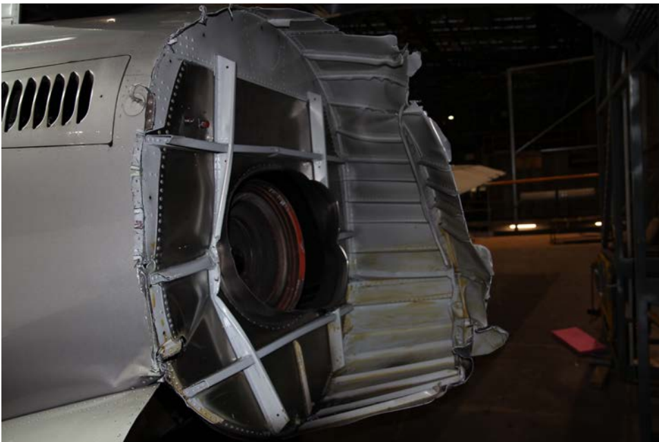
Figure 3: Damage to the tail cone of VGR aft of the APU, looking from left to right of the aircraft
