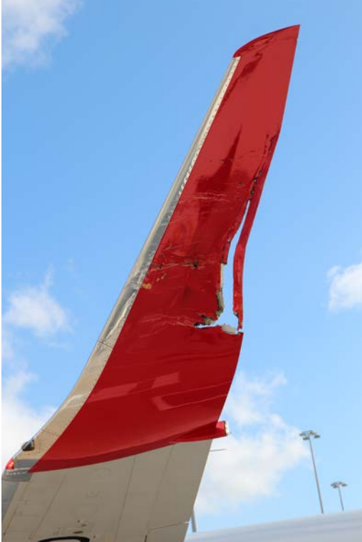
Figure 2: Damage to the left wingtip of YID
