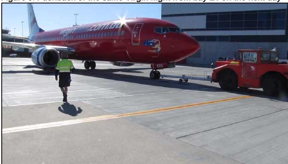
Figure 5: Pushback of the same Virgin flight from bay E1 on the next day
