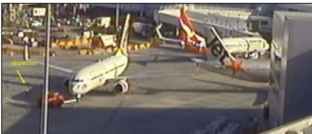
Figure 4: Screenshot of YID during pushback, 5 seconds before the collision with VGR and showing the position of the tug and the dispatcher
