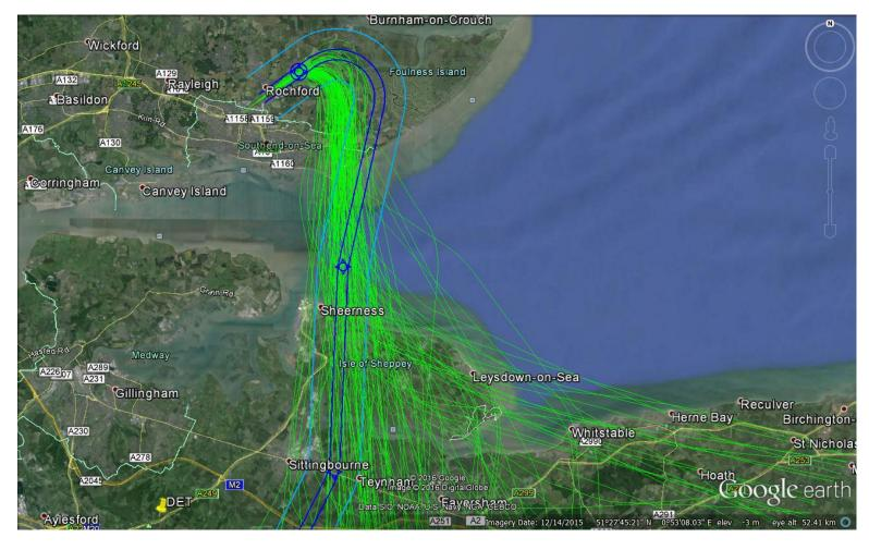
Diagram showing the anticipated maximum track dispersion (±0.2NM; dark blue) and the maximum navigation tolerance (± 1.0NM; light blue) for the EMKAD 1G SID against historic NTK tracks (green) for departing aircraft July/August 2014
