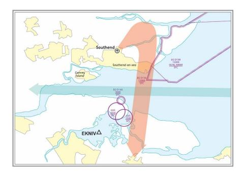
Figure F4: Schematic diagram of procedure conflicts between LSA departures (red) and LCY approach path (blue).
