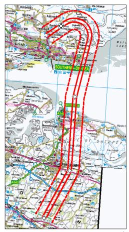
EMKAD 1G SID: Diagram showing the anticipated maximum track dispersion (±0.2NM; solid red lines) and the maximum navigation tolerance (±1.0NM; dashed red lines) overlaid on Ordnance Survey map.
