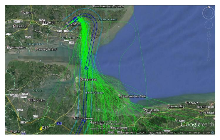
Diagram showing the anticipated maximum track dispersion (±0.2NM; dark blue) and the maximum navigation tolerance (± 1.0NM; light blue) for the EMKAD 1G SID against historic NTK tracks (green) for departing aircraft July/August 2015
