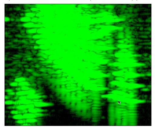
Figure 2 Example of wind farm clutter from an offshore wind farm presented on to a radar display screen.
