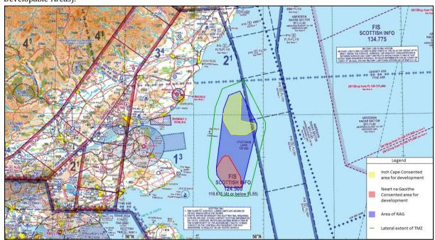
Figure 4 Design Option B of the TMZ application (the RAG is illustrated by the dark blue area emcompassing the Developable Areas).
