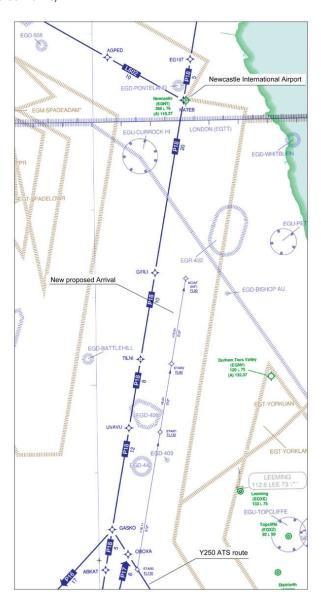
Figure 7 Chart showing proposed NIA RNAV STAR in relation to surrounding airspace
