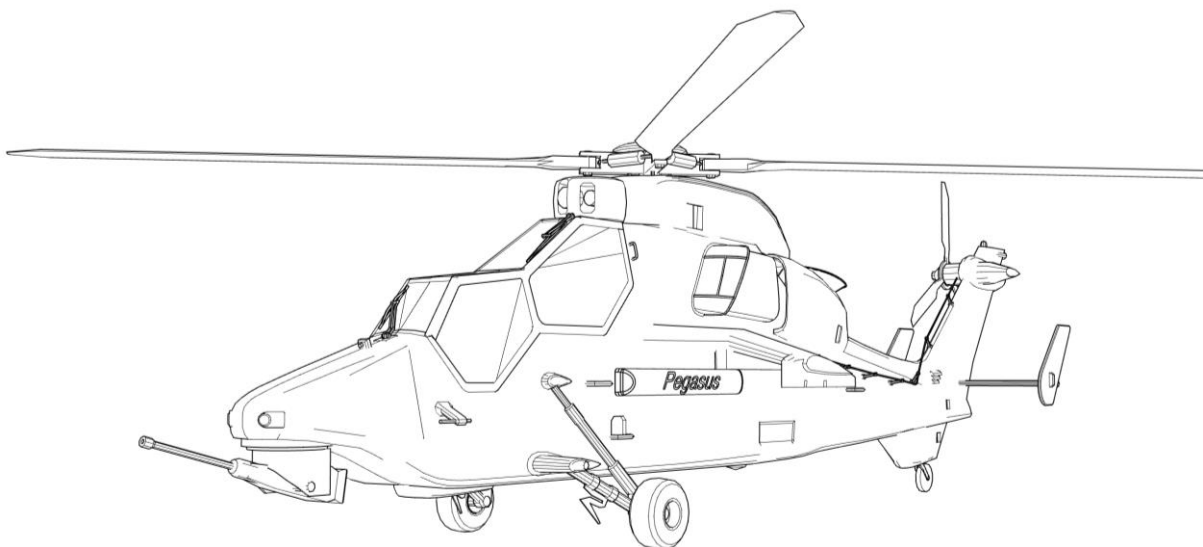
Figure 1. Pegasus installed on the Tiger Armed Reconnaissance Helicopter
