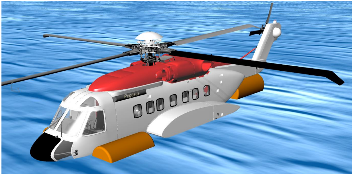
Figure 3. Post ditch prior to capsizing (2 systems fitted)
