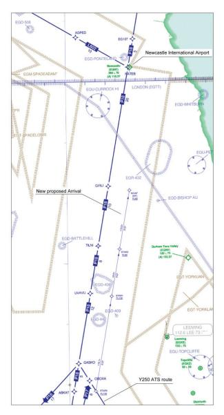
Figure 7 Chart showing proposed NIA RNAV STAR in relation to surrounding airspace
