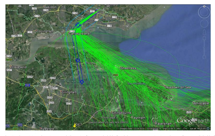
Diagram showing the anticipated maximum track dispersion (±0.2NM; dark blue) and the maximum navigation tolerance (± 1.0NM; light blue) for the EKNIV 1F SID against historic NTK tracks (green) for departing aircraft July/August 2014
