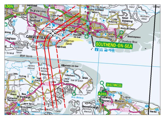
EKNIV 1F SID: Diagram showing the anticipated maximum track dispersion (±0.2NM; solid red lines) and the maximum navigation tolerance (± 1.0NM; dashed red lines) overlaid on Ordnance Survey map.
