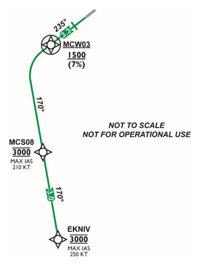
Figure C3: Schematic diagram of EKNIV 1F SID
