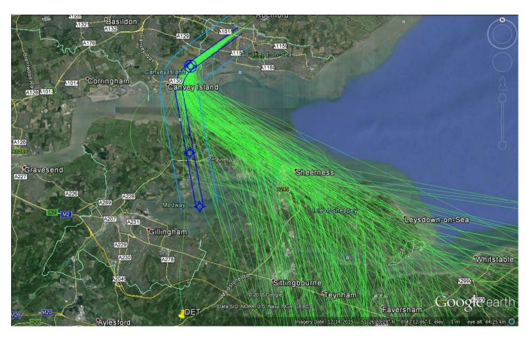
Diagram showing the anticipated maximum track dispersion (±0.2NM; dark blue) and the maximum navigation tolerance (± 1.0NM; light blue) for the EKNIV 1F SID against historic NTK tracks (green) for departing aircraft July/August 2015
