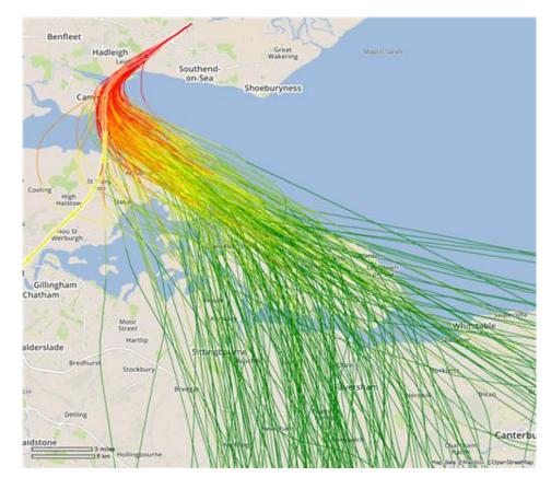
Figure C5: Colour coded climb profile of departing flights Summer 2015. [Colour coding: Below 3000ft red; 3000 – 4000ft orange; 4000 – 5000ft yellow; 5000 – 7000ft light green; above 7000ft dark green.]
