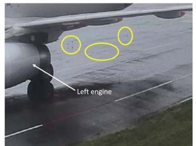
Figure 1: Foreign object debris on the ground behind the aircraft (circled)
