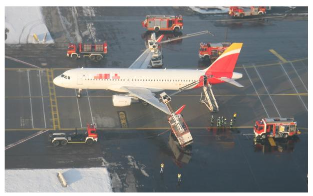
Position of the airplane and the de-icing vehicles after the collision
