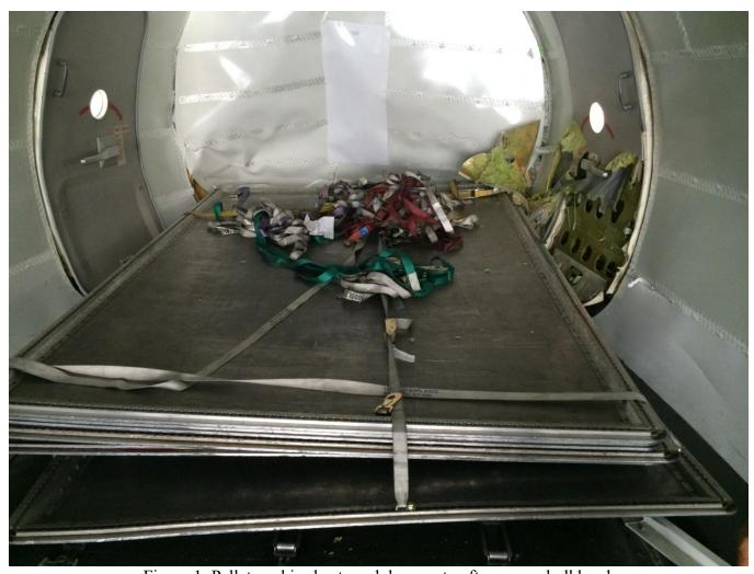
Figure 1: Pallet cookie sheets and damage to aft pressure bulkhead
