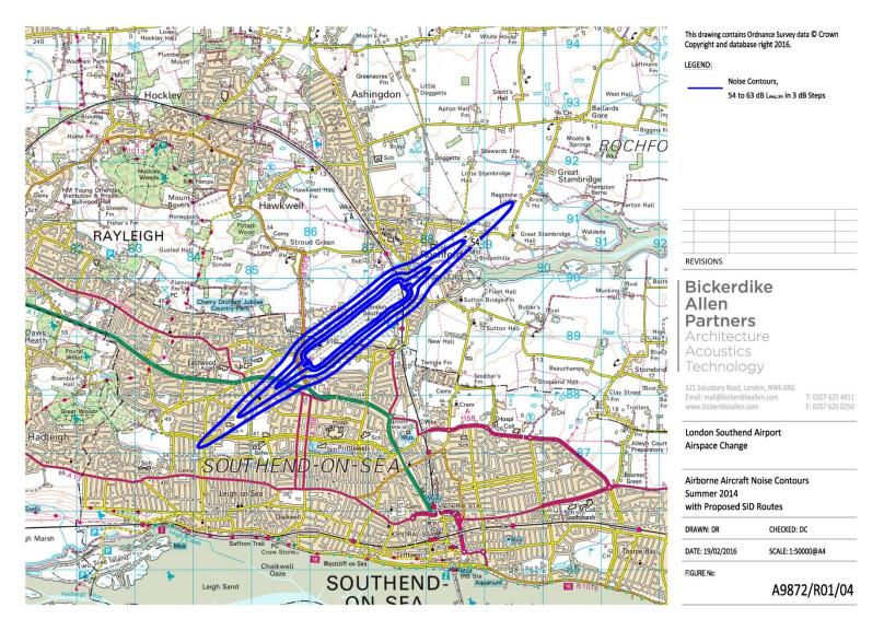
Figure 2: 2014 Noise Contour Charts adjusted to reflect SIDs.
