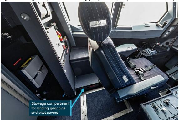
Figure 3: Stowage compartment for landing gear pins and pitot probe covers (if carried)
