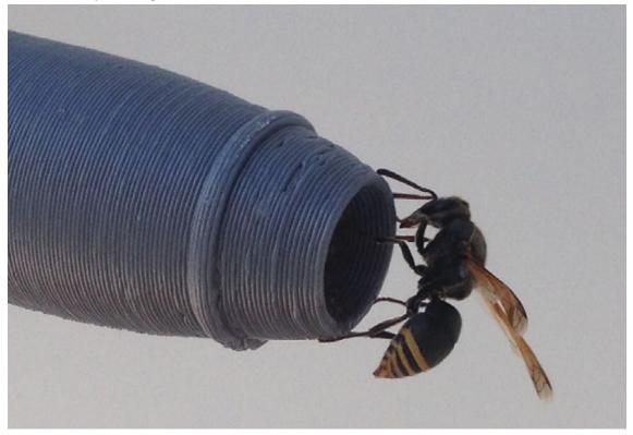
Figure 13: Female keyhole wasp (*Pachodynerus nasidens*) on a replica DHC8 pitot probe, Brisbane Airport, May 2016
